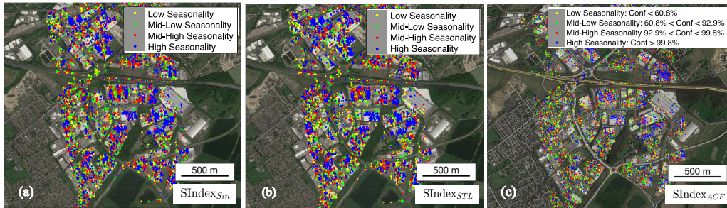
Figure 2. Dataframe of InSAR datapoints in Normanton area grouped by levels of seasonality using: (a) \text{SIndex}_{\text{Sin}} , (b) \text{SIndex}_{\text{STL}} , and (c) \text{SIndex}_{\text{ACF}} . The \text{SIndex}_{\text{ACF}} sub figure is divided into four ranges of confidence bounds. Confidence is calculated as the rejection of the Null hypothesis that the ACF value is insignificant using the standard errors under the assumption of a Gaussian source (as used by the MATLAB autocorr function). Seasonality indices \text{SIndex}_{\text{STL}} and \text{SIndex}_{\text{Sin}} are divided into four equal and sorted ranges of seasonality indexed by colour.
